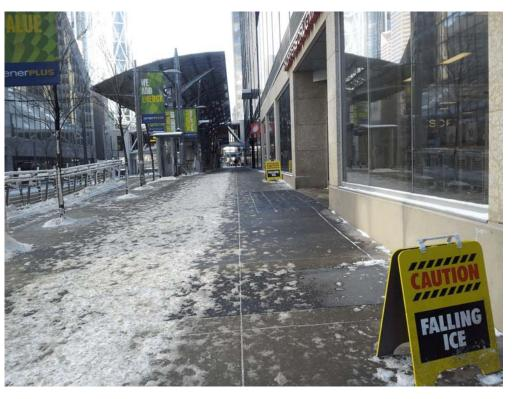
When a slab of snow or ice slides off the roof, it wafts outward a bit rather than plummeting straight down. This is because of the boundary-layer air current along the slab side of the building that pushes it outward. A wise pedestrian therefore hugs the building wall when walking along the sidewalk. The photo above shows it beautifully.
